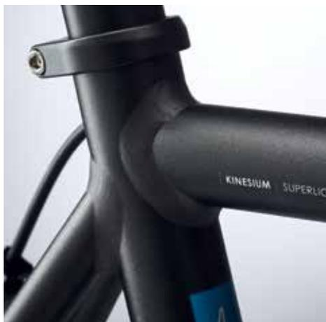
Visible welds are a defining quality of an aluminium frame, especially when, as with this anodised version of the Aithein Evo, there is no paint to hide behind. Those characteristic TIG weld pools are super neat on the Kinesis, and aside from offering a weight saving of around 100g over a painted version the anodised finish is also more durable and gives the Aithein Evo a classy look and feel.
