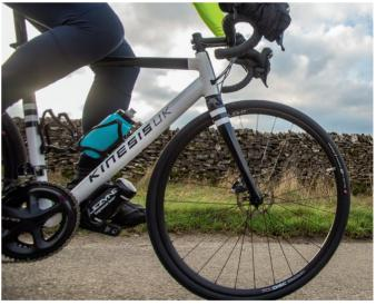
inesis UK has close ties with the global Kinesis frame manufacturer based in Taiwan, so it's unsurprising to see advanced techniques such as liquid SPF hydroforming used in its new model RTD bike. This allows tubing to be manipulated into shapes which aim to lower weight while improving strength and comfort, and an extremely rare element called Scandium has been added to the aluminium here to achieve this, creating thinner tubing in the process.
