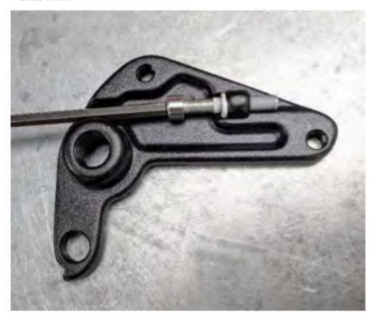
2). Prep your dropout mounting bolts with threadlock (Loctite 243).
