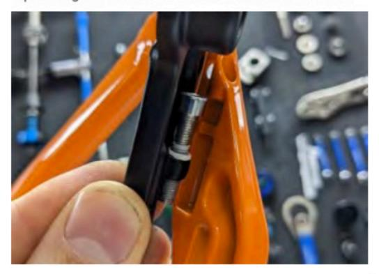
Loosely fix the dropout in place with the mounting bolts and repeat this procedure for the opposite dropout.
