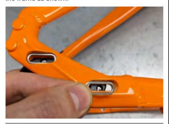
6). With the wheel in place, adjust the dropouts to the desired position by turning the captive adjuster bolts with a 4mm Allen key through the access holes as shown.
